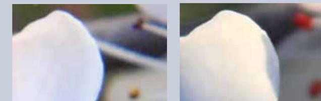
**Above** The photo (at 100% magnification) taken with a single element close-up lens (left) has chromatic aberrations around the white petal. A photo taken with a Canon 250D close-up lens (right) shows no chromatic aberrations at all.
